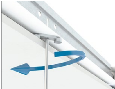
Mountening of locking clip with screwdriver.
