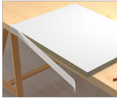
3. Align 5 mm overlap on front and press.
