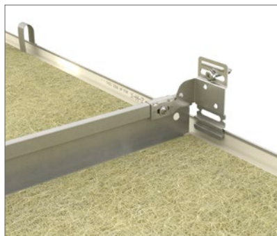
To secure the squariness of the Rockfon System T24 X it is recommended to use a wall bracket on every main runner and every second cross tee.
